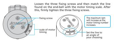
In order to prevent failure, adjust the motor timing to 60° or below to match the settings in the ESC.
