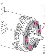
Use the four screws other than the screw holes to fix the motor mount, and fix the motor and spacer with the attached screws
