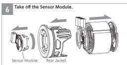
Turn the Sensor Module and pull out it so that the protrusion on the outer circumference matches the recess on the inner circumference of the rear jacket.
